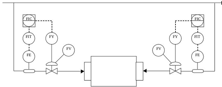
**FIGURE 5 Individual water flow instrumentation and controls for a semi-autogenous grinding mill**
