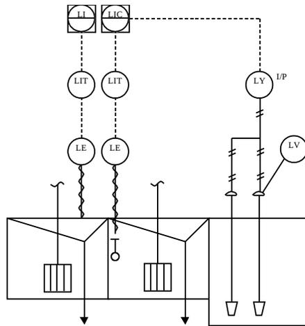
**FIGURE 3 Flotation bank froth height instrumentation and pulp level instrumentation and controls**
