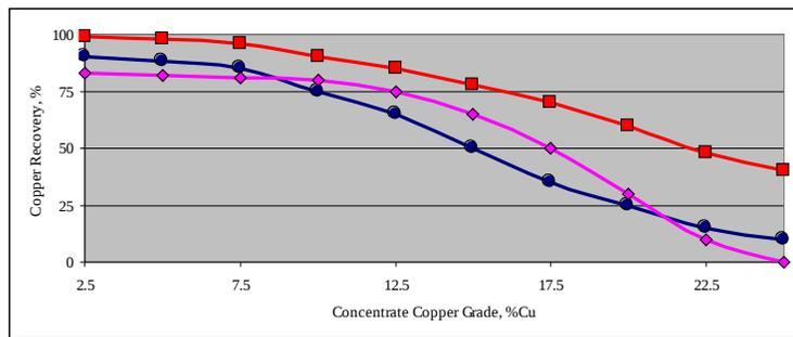
**FIGURE 7 Rougher flotation response curve of three different ore-types and particle size distributions**
