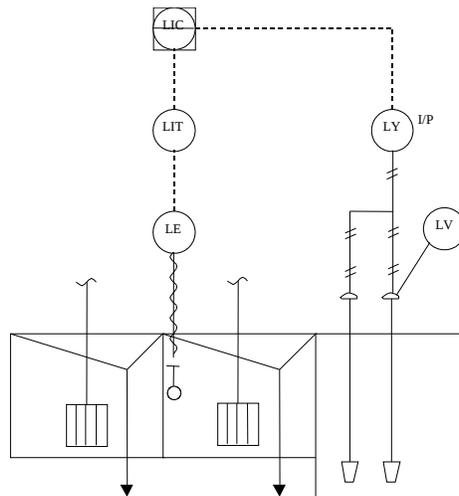
**FIGURE 2 Typical flotation bank pulp level instrumentation and controls**
