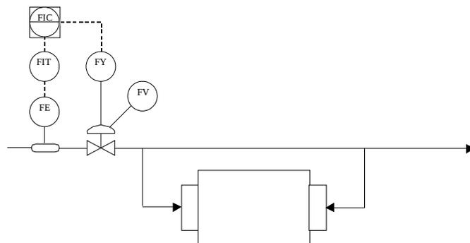
**FIGURE 4 Total water flow instrumentation and controls for a semi-autogenous grinding mill**
